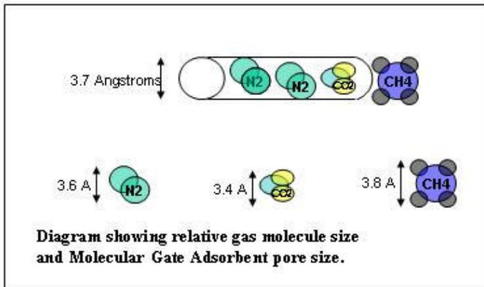
Figure 3: Schematic of size separation within the Molecular Gate Adsorbent.
