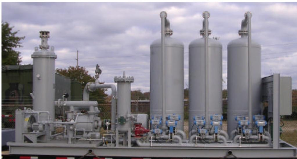
*Figure 6: A SPEC plant used to treat smaller flows*
