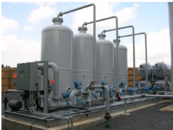
Figure 4: Typical installation for a 2-4 MM SCFD Molecular Gate nitrogen rejection unit
