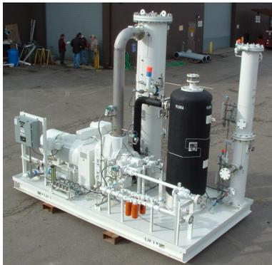
*A Guild packaged biogas feed compressor*
