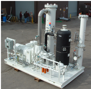
A Guild packaged biogas feed compressor
