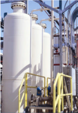
Figure 5. A Molecular Gate Adsorbent-Based System for CO 2 removal
