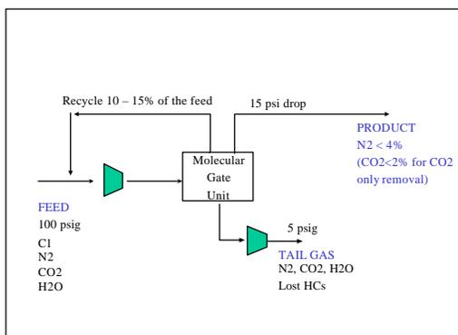
**Figure 3.** Block flow diagram of the Molecular Gate process
