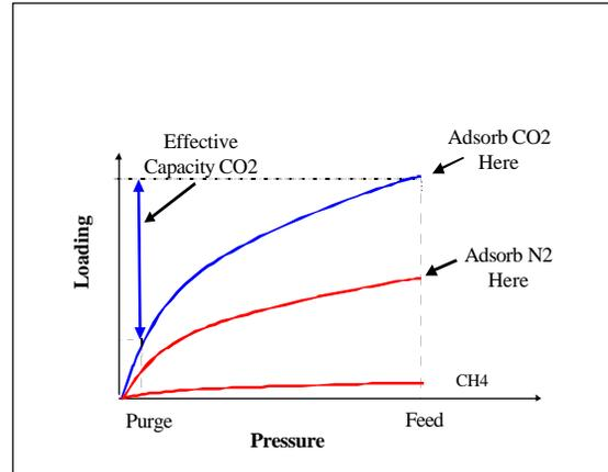
**Figure 2** Generic isotherm for adsorption and PSA pressures
