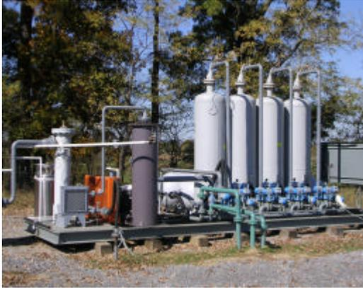
**Figure 5.** A small 1 MM SCFD unit designed to upgrade CMM
