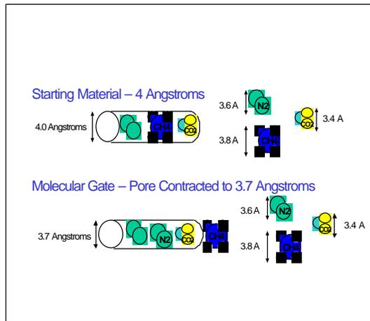
**Figure 1.** Schematic view of the Molecular Gate pore size and relative molecule size
