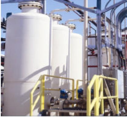
**Figure 4.** *Tidelands Oil Production Company CO<sub>2</sub> removal unit*
